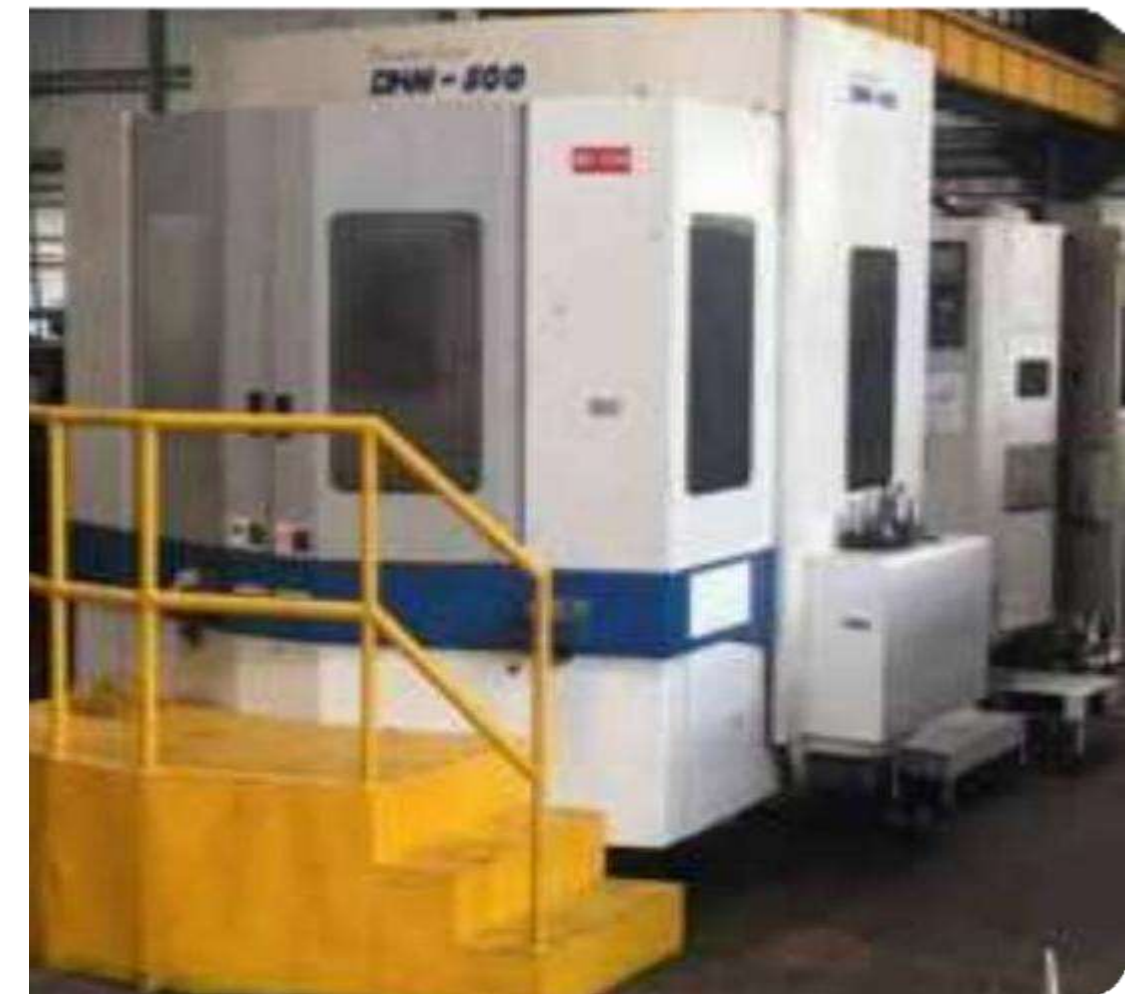
DOOSAN DHM 800 With Probing Operating Spec : 1200x1200x900mm Pallet Size : 800x800mm ATC : 90Nos
