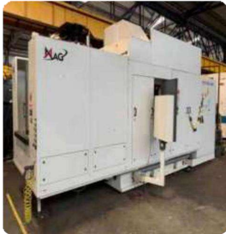
MAG SPECHT - 500X 5 th Axis Operating Spec : 800x800x750mm Pallet Size : 500x500mm ATC : 108Nos
